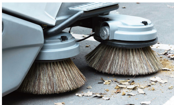
Panel button control on the side brush and rolling brush up and down
